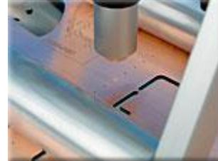
with the measuring system. The 1600 x 1200 pixel USB 2.0 camera provides for 900x or 1,350x final magnification on a 17" screen.
