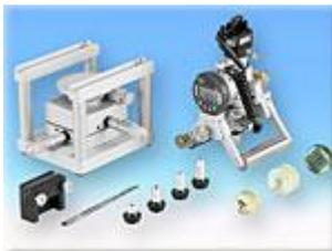
The MST stand provides a secure position on drums or flat material for depth measurement. An additional five millimetre X-adjustment at high magnification allows feed motion between the focal planes, when they can no longer be covered by the field of vision. In addition to visualisation the Metric Standard or Metric MT
