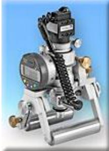
The ideal aid for depth measurement. The digital dial gauge measures the distance between two focal planes for no-contact measurement of hole depths in circuit boards or cell depths on anilox rollers and intaglio cylinders. The measurement should be accomplished at very high magnification to limit the depth of field - a possible source of error. For this reason 20x and 30x lenses are included
