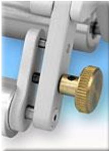
Important for optimum readings: Always focus the top and bottom focus level from the same side. This is the only way to ensure elimination of inaccuracies in the measurement resulting from a slight backlash. Here the coaxial illumination directly through the lens plays a significant role. This light guidance is the only feature that allows exact recognition of the focal planes. The fine focusing mechanism can be pushed to the side for quick adjustment. An LED ring light is
